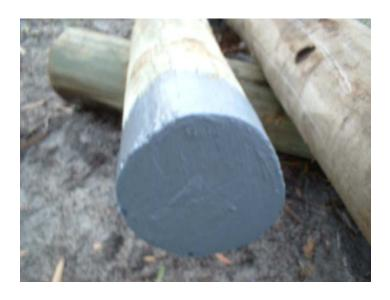
TERM-seal Multi-Purpose Passive or TERM-seal Multi-Purpose Active coatings are the perfect answer to treating posts, poles, bridge timbers, wharf timbers or any type of timber where termites and moisture can damage timbers.
