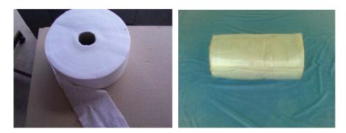
TERM-seal Reo-sheet is supplied in 500mm x 160m rolls and is used as covering to back-filled wall applications of TERM-seal Multi-Purpose coatings to prevent foreign intrusion in the fill
