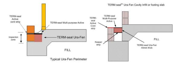
TERM-seal Ura-Fen is the perfect termite proofing system for cavity perimeters in all types of slab construction
