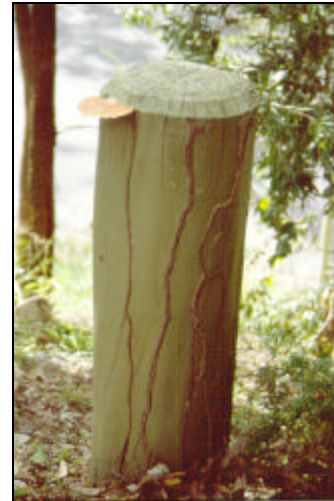
Figure 7. Microcerotermes sp. attacking painted timber decayed by the fungus Pycnoporus coccineus .
