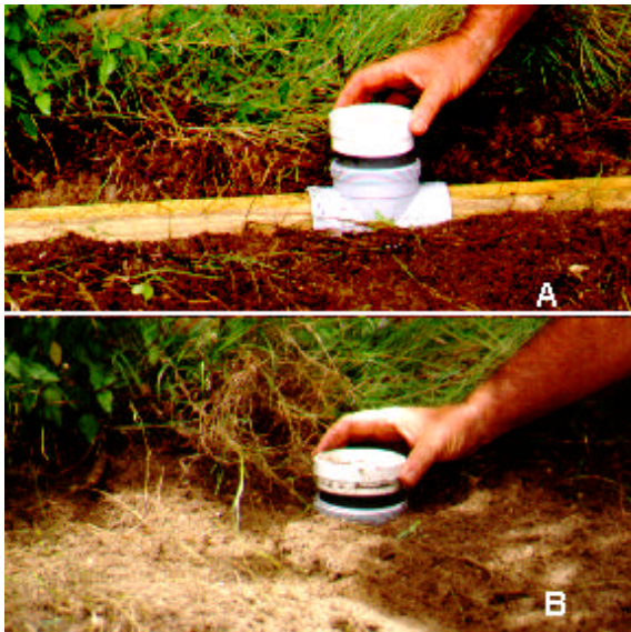
Figure 5. Termite aggregation station with plastic-“T” piece and timber:
