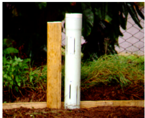
Figure 4. Termite aggregation station with slotted-PVC-stormwater pipe and timber prior to installation.
